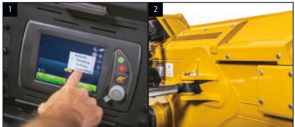
Grade-control system includes Topcon 3D-MC<sup>2</sup> components.
