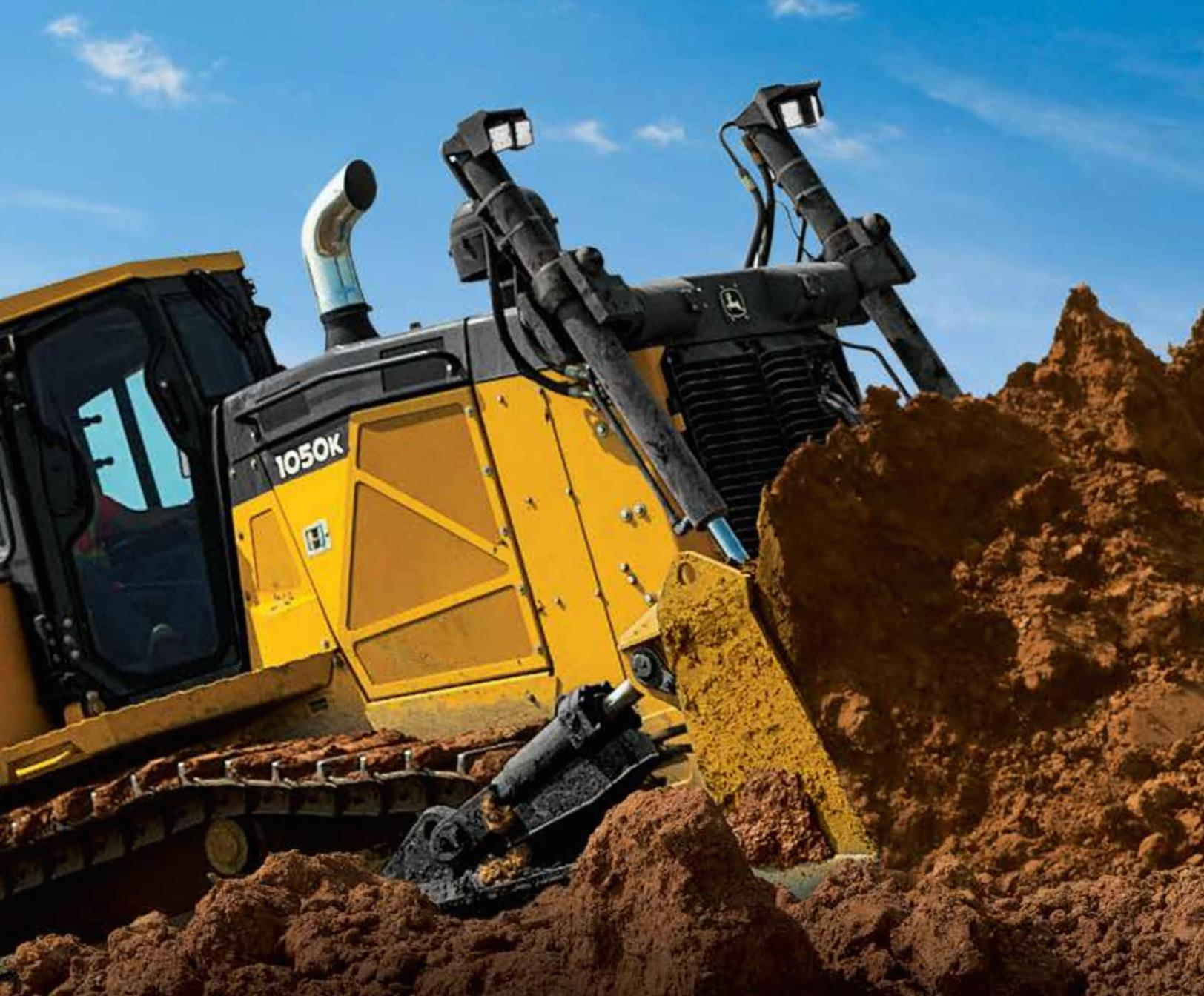
2. Independent track control speeds up or slows down each side — for smooth, full-power turns.
