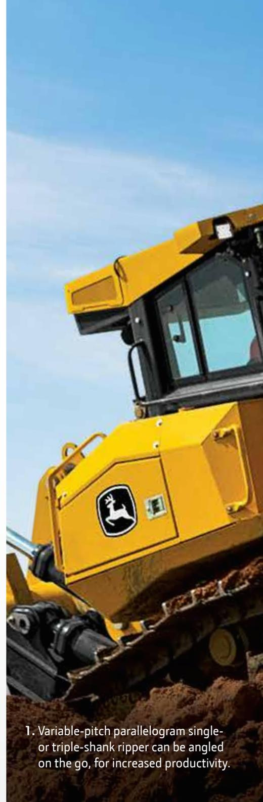
1. Variable-pitch parallelogram single- or triple-shank ripper can be angled on the go, for increased productivity.
