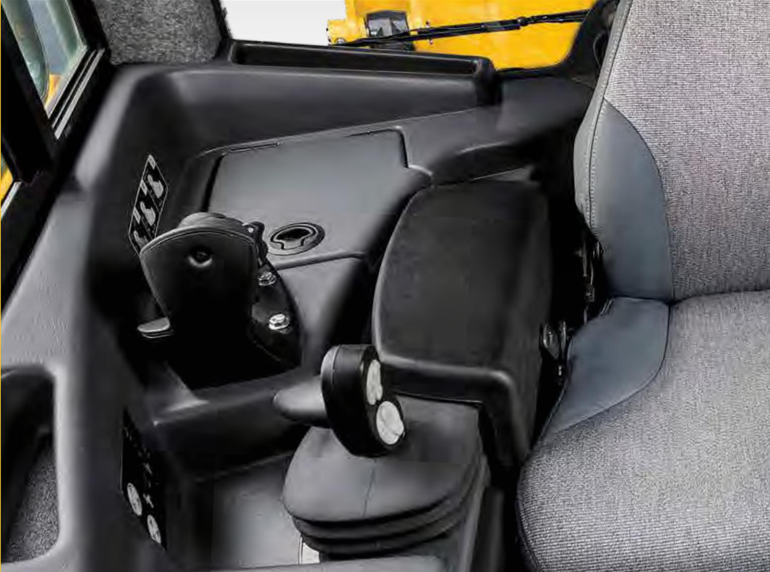
1. Beyond cup holders and cooler storage, there are plenty of places to store stuff. If you're running a grade-control system, the lockable in-dash compartment is ideal for end-of-day storage (or permanent placement) of the monitor. Overhead radio and storage console includes a 12-volt electrical outlet for powering a cell phone or an iPod®.
