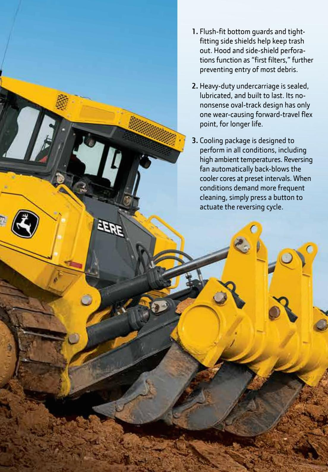
1. Flush-fit bottom guards and tight-fitting side shields help keep trash out. Hood and side-shield perforations function as “first filters,” further preventing entry of most debris.
