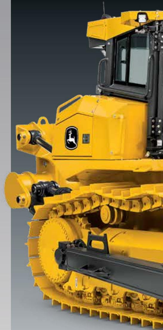
1. Large hinged doors provide ample access for easy everyday checks and periodic maintenance. Daily service is limited to hydraulic-oil and engine-oil and -coolant levels. Operator station tilts a full 70 deg. in only minutes, for wide-open drivetrain-component access.
